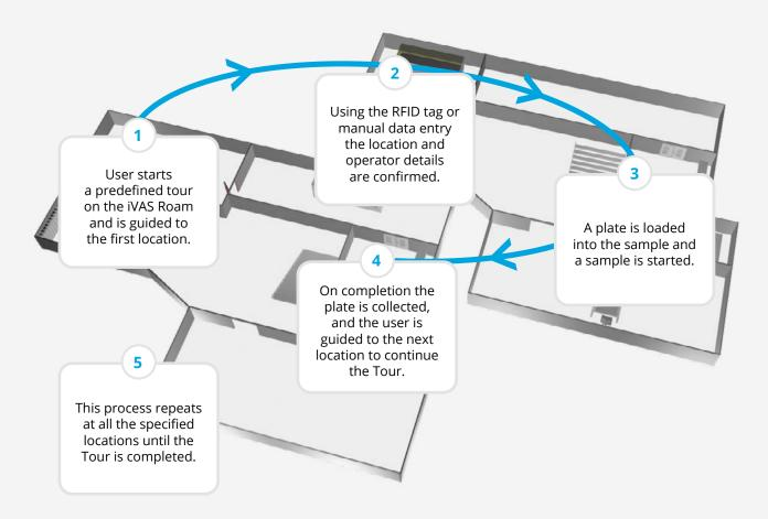
Each Tour is easily configured via the Manager App using an intuitive user interface, which supports the ordering and dragging of locations to craft the exact sequence desired for the sampling process. Tours are then saved directly to the unit, ensuring a seamless transition from planning to execution. Multiple Tours can be configured and saved to the same iVAS Roam; these can also be duplicated to other units.
